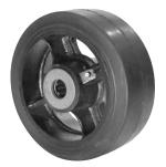
Rubber tread wheels are constructed by molding high quality rubber to cast iron cores. All mold-on rubber wheels are floor protective, provide long tread life, are quiet in operation and are highly resilient. These wheels are suggested for use on all types of floors and numerous applications.
